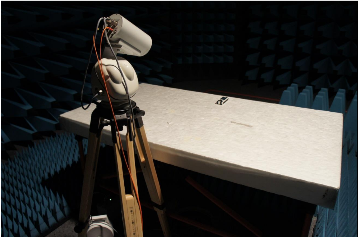
Picture 6: Test setup radiated immunity test
