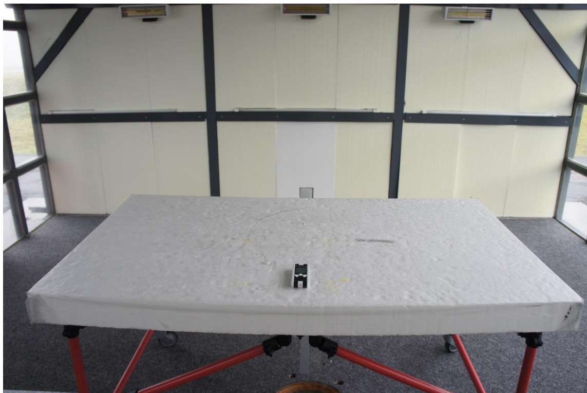
Picture 4: Test setup radiated emission
